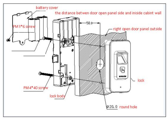
Remove the battery cover and batteries. Pass the wire through the 20mm middle hole & connect it to the lock body connector. Install the reader and lock body using the screws provided, and as shown in the diagram, if door thickness is less than 15mm you will have to shorten the longer 4\*40 screws. For 12mm thick door shorten it by 3mm.
