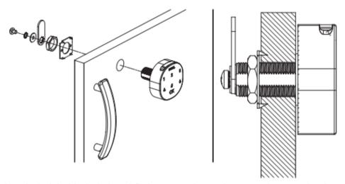
Place the lock inside the hole and fit the accessories one by one as shown on the picture above.
