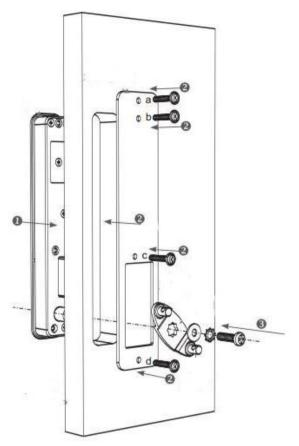
Place the lock inside the cutout and fit the accessories one by one as shown on the picture.
